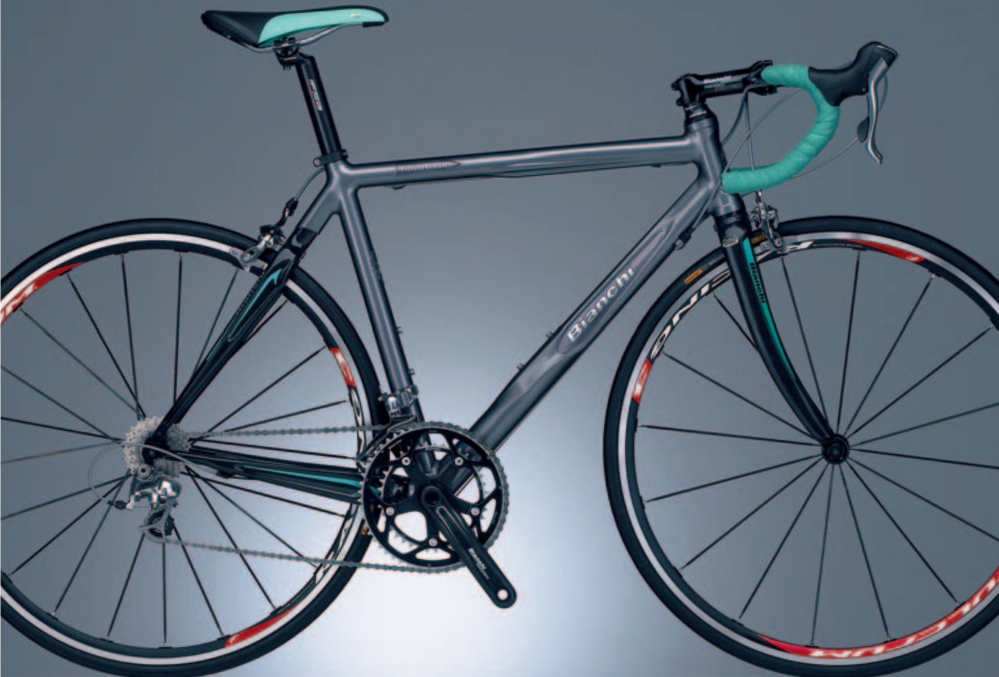
FRECCIA CELESTE HC MIX 105/ULTEGRA, Y6B20, COLOUR KT - GROUP SHIMANO 105/ULTEGRA, HANDLEBAR ITM MILLENNIUM WINGSHAPE CARBON, STEM ITM FORGED LITE CARBON, SEATPOST FSA SL-K CARBON, CRANKSET BIANCHI COMPONENTI CARBON W. ALU SPIDER, WHEELS FULCRUM RACING 3. ALSO AVAILABLE IN COLOUR CX AND AS FRAMESET (X6B03).
