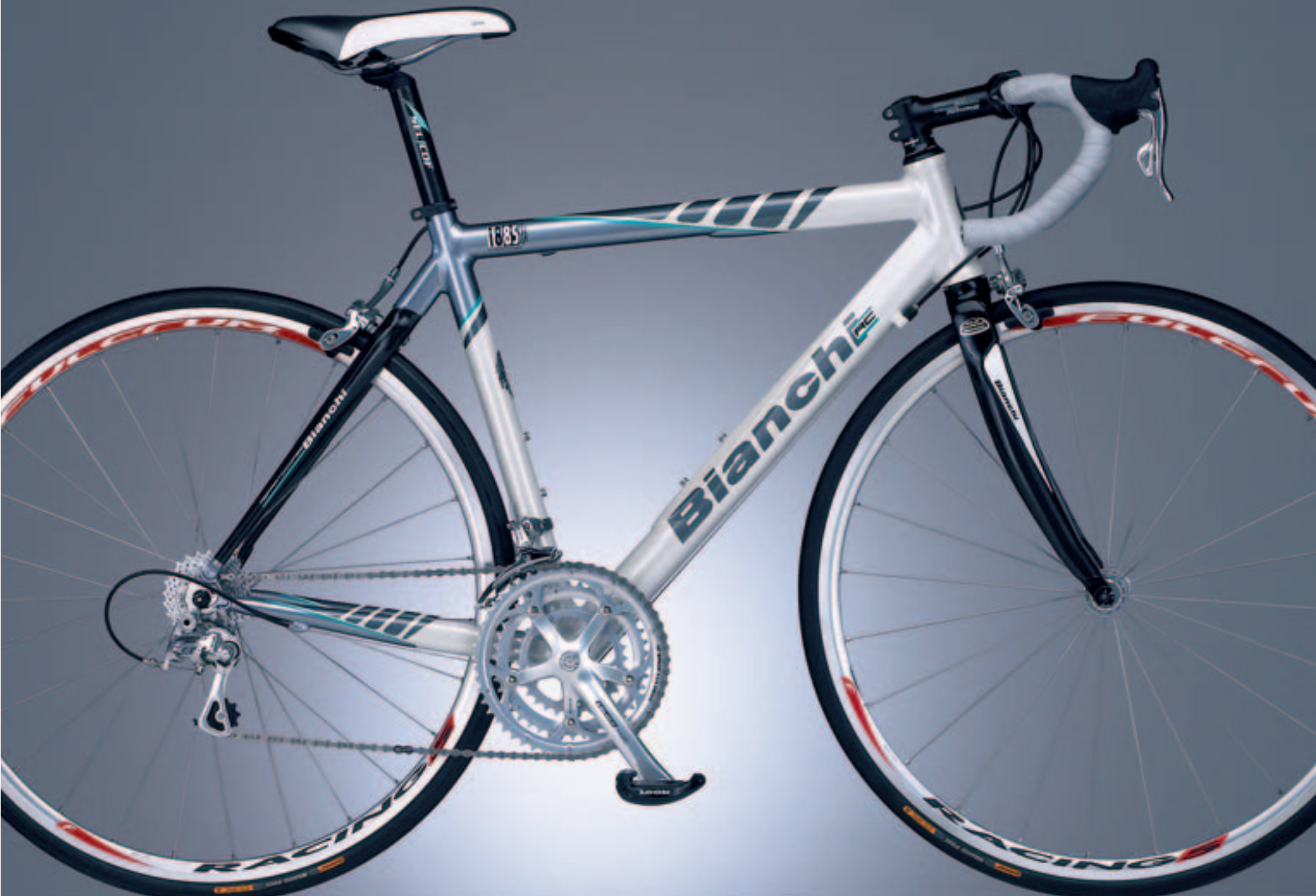
1885 TB HYDRO CARBON CENTAUR TRIPLE, Y6B07, COLOUR WG - GROUP CAMPAGNOLO CENTAUR, HANDLEBAR ITM LITE LUXE WINGSHAPE, STEM BIANCHI COMPONENTI 3-D FORGED ALLOY SUPER OVER, SEATPOST SELCOF 91A CARBON, CRANKSET CAMPAGNOLO VELOCE TRIPLE, WHEELS FULCRUM RACING 5. ALSO AVAILABLE WITH COMPACT 50/34 RINGS (Y6B08), IN COLOUR CZ AND AS FRAMESET (X6B08).
