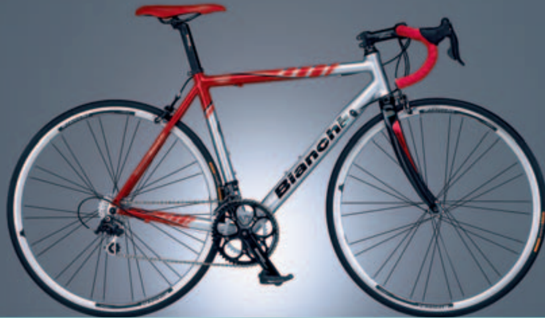
VIA NIRONE 7 XENON COMPACT, Y6B14, COLOUR SL - GROUP CAMPAGNOLO XENON, HANDLEBAR ITM 330 SUPER OVER, STEM BIANCHI COMPONENTI 3-D FORGED ALLOY SUPER OVER, SEATPOST BIANCHI SP-151, CRANKSET FSA CFJ-215 COMPACT, WHEELS BIANCHI COMPONENTI RACING. ALSO AVAILABLE WITH TRIPLE 52/42/30 (Y6B15) AND IN COLOUR CY.
